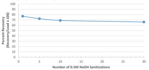
**Figure 1**: LigaTrap® Prepacked Column alkaline stability. Load: <u>40 mg IgG /mL Resin</u>. 0.5M NaOH contact time of 20 minutes per cycle.
