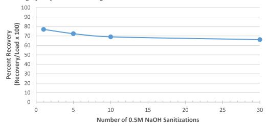
**Figure 1**: LigaTrap® Prepacked Column alkaline stability. Load: <u>15 mg IgM/mL Resin</u>. 0.5M NaOH contact time of 20 minutes per cycle.
